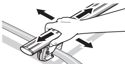
(EN) Test the anchoring: the crossbars should not move. Tighten more if necessary.
